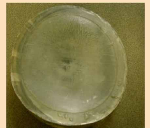
Cut off billet end, coated with boron nitride.
