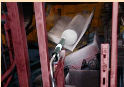
Automatic Boron Nitride dry powder coating of aluminium billets without human intervention
